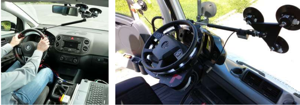
Illustration 3: Steering Robot installed in Passenger Car (left) and Commercial Vehicle (right)
