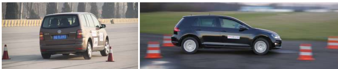
Illustration 1: Examples for the use of VEHICO Robots: Double Lane Change and Circle Driving
